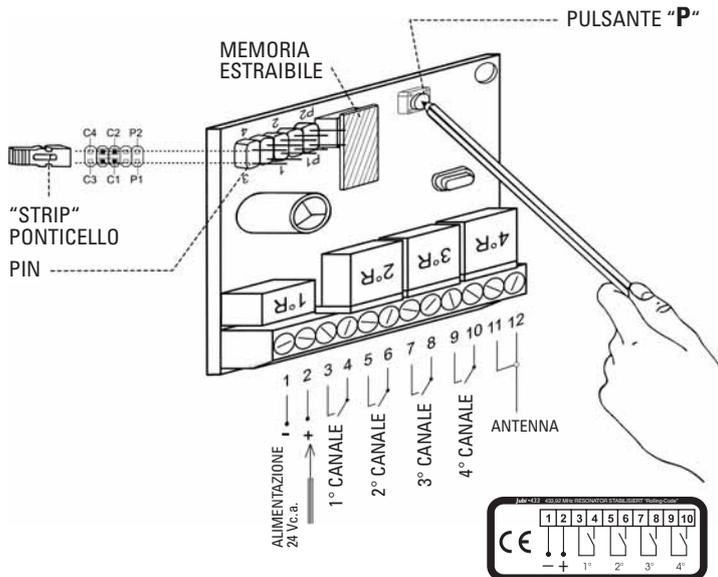
RICEVITORE RADIO AD INNESTO Jubi•433 - 2 CANALI - RISUONATORE STABILIZZATO, 433,92 MHz, AD AUTOAPPRENDIMENTO, “ROLLING-CODE”
